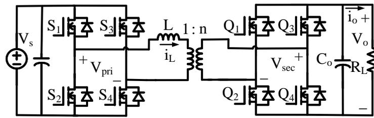
Figure 1. Isolated DAB converter.
