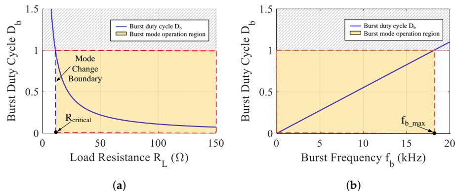
**Figure 8.** (a) Critical load value  $R_{critical}$  for mode change condition; (b) the burst-mode duty cycle  $D_b$  versus burst frequency  $f_b$ .
