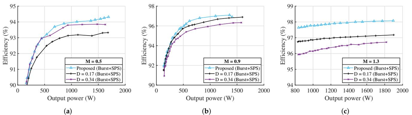
**Figure 18.** Efficiency measurement comparison for (a)  $M = 0.5$  (b)  $M = 0.9$  (c)  $M = 1.3$ .
