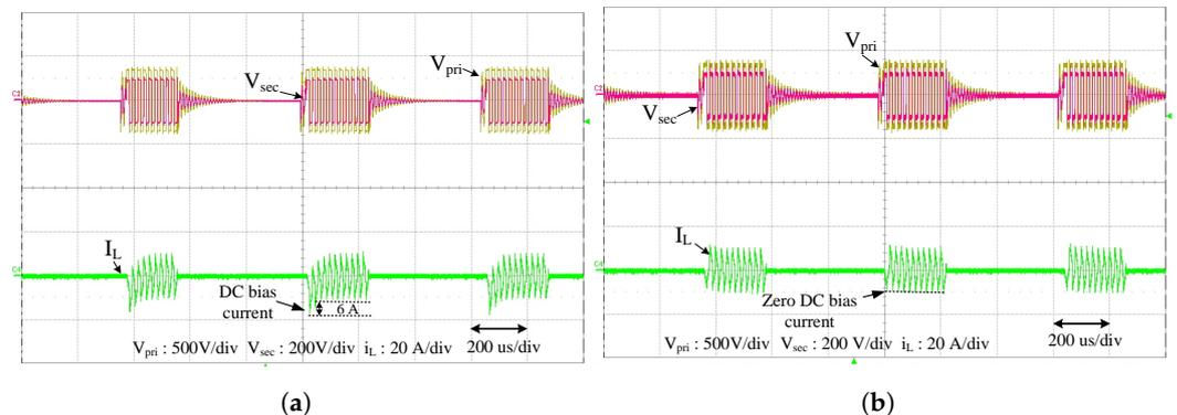
**Figure 13.** Experimental waveforms of DC bias current elimination for boost operation mode: (a) conventional burst-mode and (b) proposed burst-mode.
