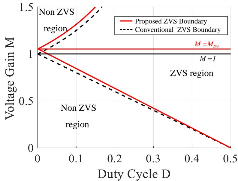
Figure 6. ZVS condition boundary with the new ZVS condition.
