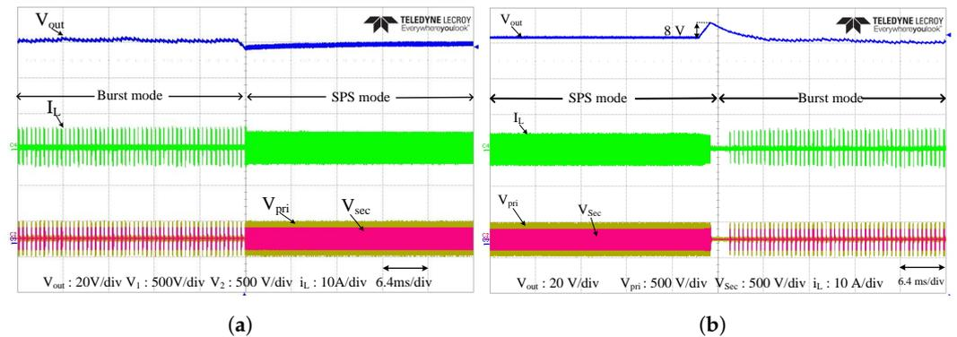
**Figure 17.** Experimental waveforms of the mode switching (a) from burst-mode to normal mode and (b) from the normal mode to burst-mode.
