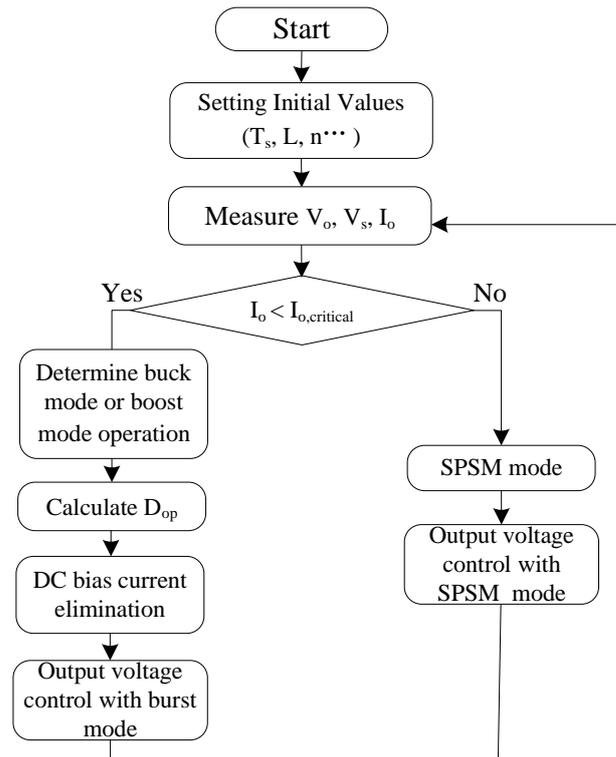
Figure 10. Proposed burst-mode control flowchart.
