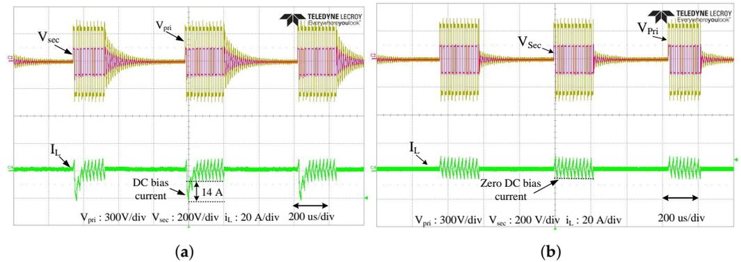
**Figure 12.** Experimental waveforms of DC bias elimination for buck operation mode: (a) conventional burst-mode and (b) proposed burst-mode.
