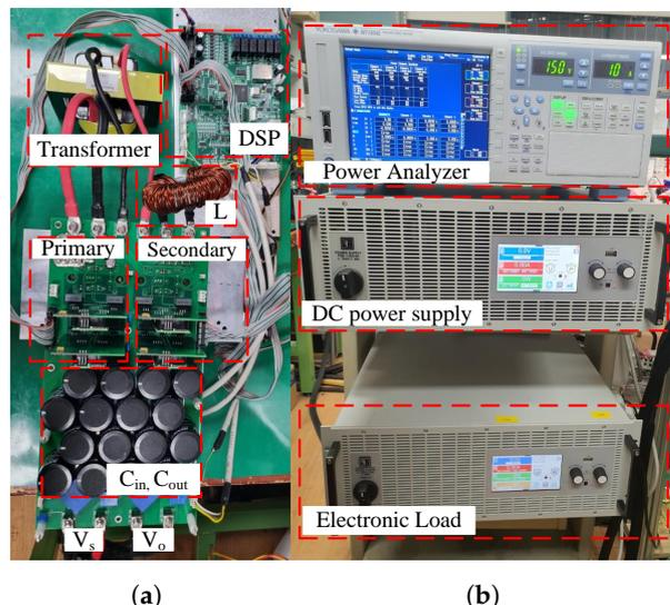
Figure 11. Experimental setup: (a) prototype DAB converter; (b) DC power supply, electronic load, and measurement equipment.
