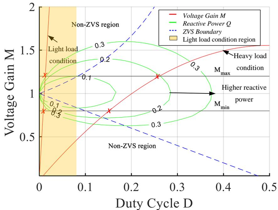
Figure 3. ZVS condition and backflow power for different voltage gains and load conditions.
