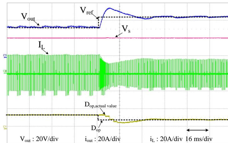
**Figure 15.** Experimental waveforms of the proposed burst-mode control when  $V_{ref}$  changes from 90 V to 120 V.
