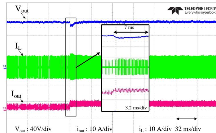
**Figure 16.** Experimental waveforms of DAB converter of the proposed burst-mode control when load changes from 80  $\Omega$  to 40  $\Omega$ .
