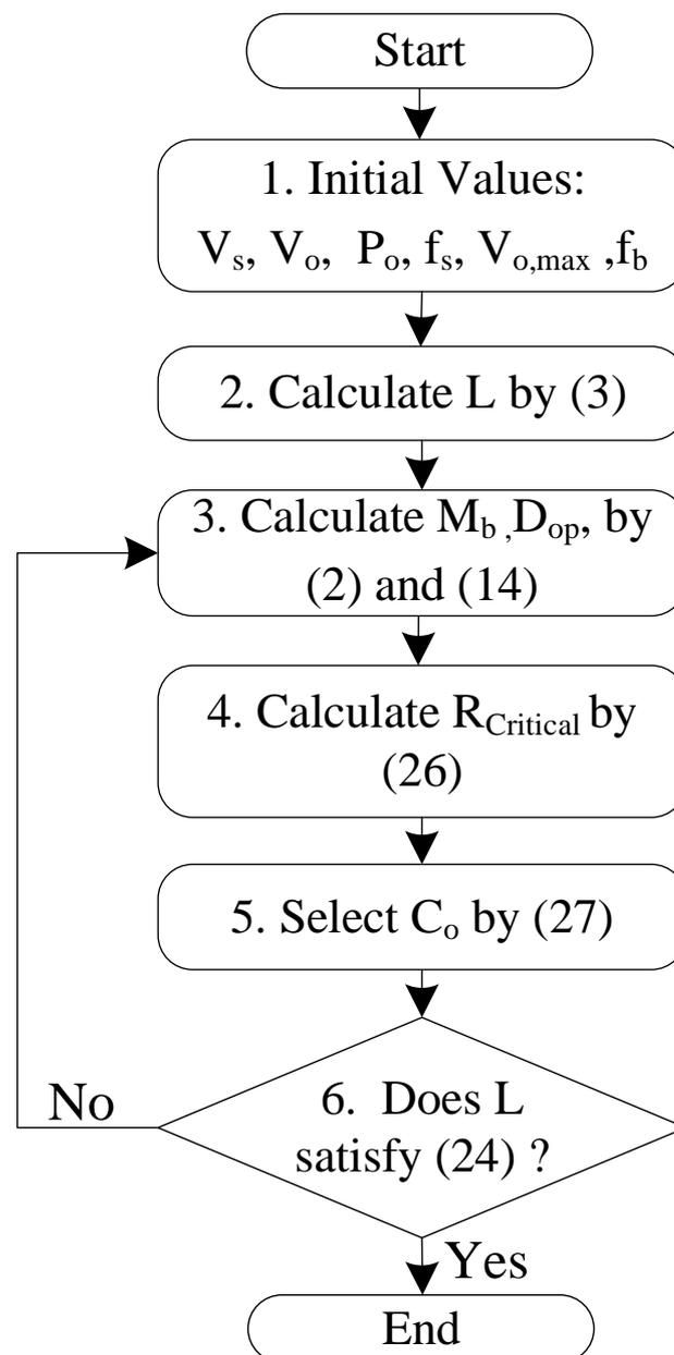
**Figure 9.** Design procedure of the proposed burst-mode method.
