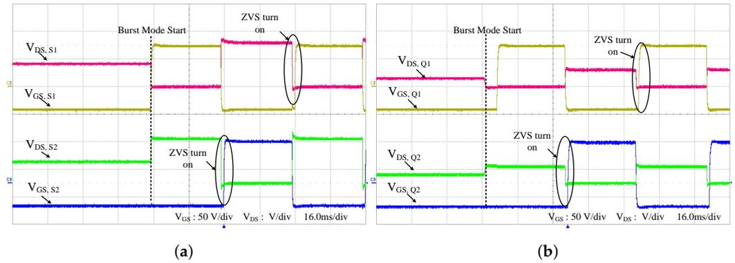
**Figure 14.** Experimental waveforms for ZVS of (a) primary side and (b) secondary side.
