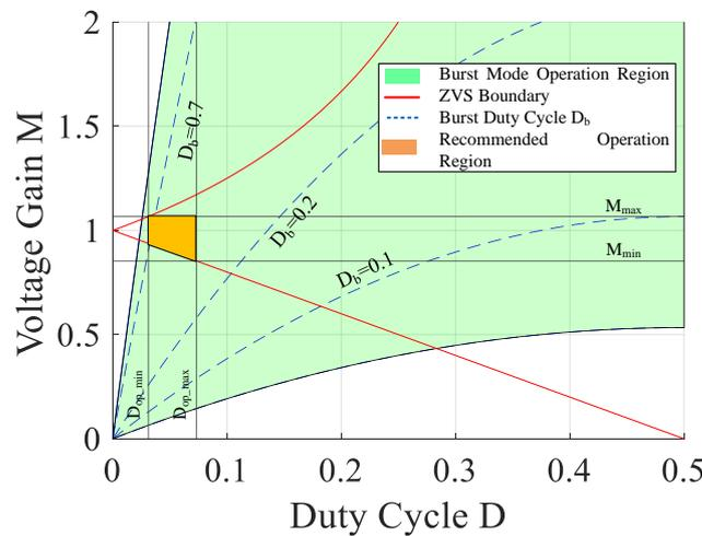
Figure 5. Determination of the operation region for proposed burst-mode control.
