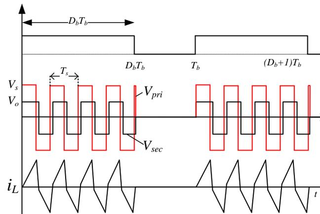
Figure 4. Burst-mode operation waveform.
