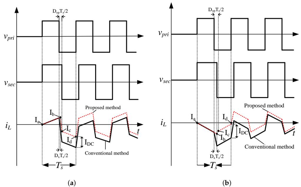
Figure 7. DC bias elimination key waveforms of the proposed burst-mode control in (a) buck operation mode and (b) boost operation mode.
