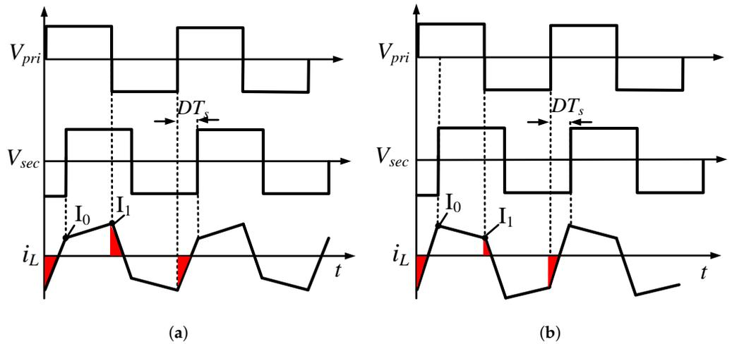
Figure 2. Key operation waveforms of the DAB converter with SPS modulation control: (a) buck operation mode and (b) boost operation mode.
